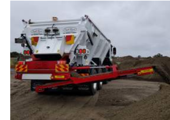
• Pivoting Side Conveyor Extends from 1.5m to 3m past the RH side of the body
