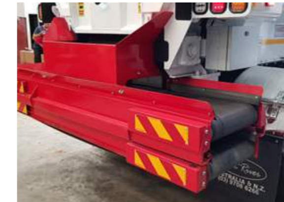
• Extendable Side Conveyor (horizontal) Extends out 1.5m past the RH side of the body
