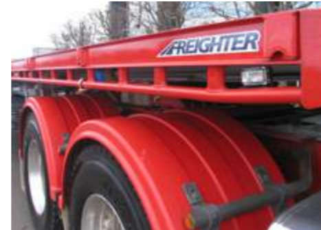
• 25mm NB pipe tie rails
